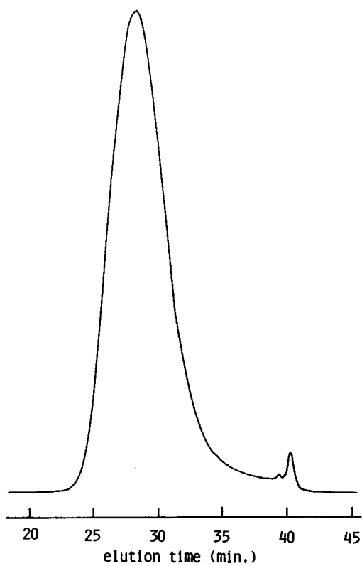
Fig. 2. A typical GPC chart for PET prepared by melt polymerization.
